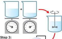
Measure the base material and catalyst by weight as specified for the grade selected. Mix the components thoroughly. Vacuum-degas the silicone mixture to remove air
