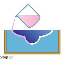
Secure the master model to the mold so the base is flush with the base material. Pour silicone into the cavity between the base and master model. Cure the silicone according to the specified conditions.
